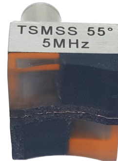
Extra Miniature Single Shear 55° with \phi 6.3mm Crystal in tandem 5MHz with Lemo 00 Connectors
