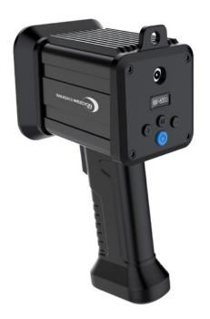
The Iris series of portable LED UV inspection lamps feature 3 powerful UVA (365 nm) LEDs, plus a convenient white light LED to switch between fluorescent inspection and flaw location quickly. The smooth, large beam of this hand-held UV lamp makes it a useful tool whether in the field or on a bench. The laser pointer makes it possible to pinpoint the crack location on big parts, identifying locations amongst operators. All lamps are equipped with UVA filters.
