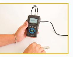
With more than 75 years of world-wide experience in ultrasonic design, Danatronics is pleased to welcome our EHC-03 to our corrosion thickness gage family. The EHC-03 is designed to accurately and non-destructively measure metal structures subject to corrosion.
