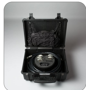
Transport Case 3: Contains two 8m long Signal cables, reference plate, encoder plates and a rucksack.
