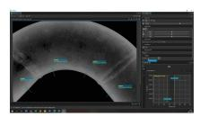
With the Advanced Wall Thickness Tool of D-Tect X, you can easily analyze the wall thickness at one or more points along the walls of a pipe.
